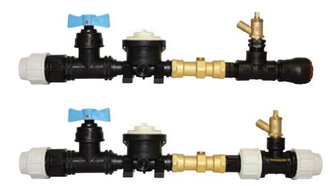
Connection from the manifold for each individual supply requires several components to be included to meet water company requirements and regulations. Water meter mounts are supplied with a full flow cap to enable commissioning, prior to fitting the water meter. The stop valve and concentric water meter housing are supplied in kit form including all the necessary components to meet current regulations, and are fully WRAS compliant.
